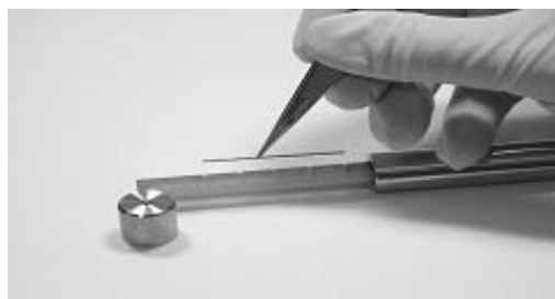
Figure 6: Removing RAPID Strand from spacing jig
